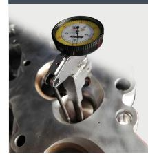
Device to insert on a pilot shank after seat machining, to display the runout value. The gauge turns around the pilot and the runout value must be read on one device rotation.
