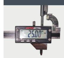
Digital display micrometer allowing to measure the current diameter position of the tool tip, and to implement it into the machine to set its diameter reference.
