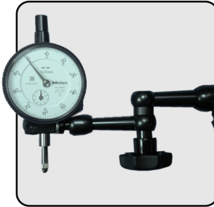
To machine the seats to the same depth position. Metric version.
