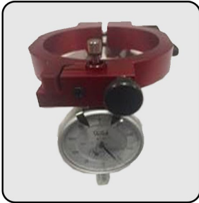
Lower spindle indicator original design. (US market only)
