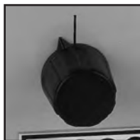
Vacuum control knob has 3 settings — continuous, hold and release
